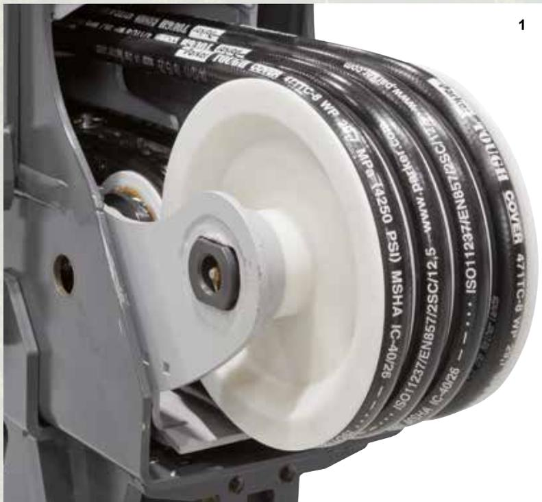
**1. Internal hose routing.** Cranab was the first with this obvious solution – well-designed internal hose routing that protects the lines. The development has given Cranab the opportunity to design products with hoses that can operate at higher pressures.
