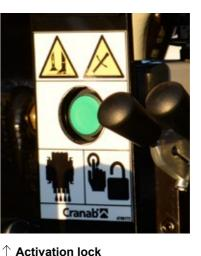
Control more than the crane Start and stop the truck's engine and control its rpm.
