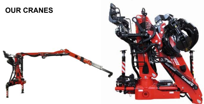
RZ13 • RZ13TR • RZ15 • RZ16XP A perfect choice for material handling and recycling. Modern, strong and flexible cranes with maximum reach between 7.9 and 10.5 metres. Available as a single or double telescope crane and in several versions. The RZ16XP has a powerful working pressure of 31.5 MPa.
