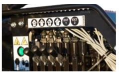
Support leg valve Electrically/manually operated. 4 sections suitable for single-circuit, dual-circuit and LS systems.
